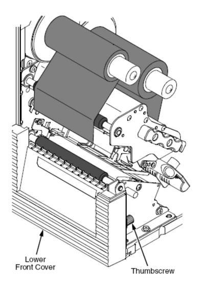
Remove the thumbscrew that secures the lower front cover to the printer. Slide the cover to the left (toward the electrical half of the printer) to remove it.
